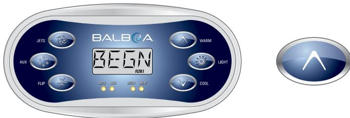
The hour will flash. Press LIGHT to advance to minutes. (Reminder: Since filtration will be set for 24 hours, the start/stop time is not important.)
