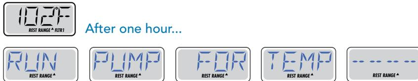
**Rest Mode:** The Screen will display RUN PUMP FOR TEMP if the filtration pump has not run for over 1 hour.
