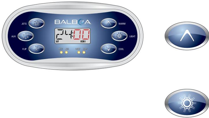
If needed, adjust the minutes to zero by pressing TEMP.
